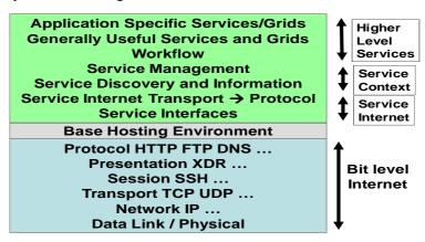
Figure 1.13 Layered architecture for web srvices and grids
