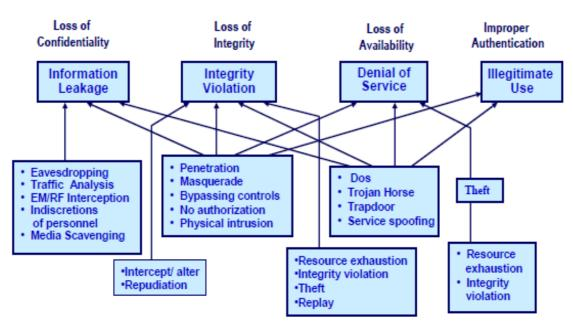
Figure 1.20 Various system attacks and network threats to cyberspace.
