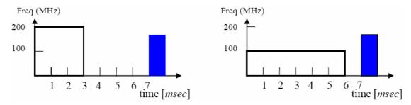
**Figure 1.23 DVFS technique (right) original task (left) voltage-frequency scaled task** (Courtesy of R.Ge, et al, "Performance Constrained Distributed DVS Scheduling for Scientific Applications on Power-aware Clusters", *Proc. of ACM Supercomputing Conf.*, Wash. DC, 2005 [16].)
