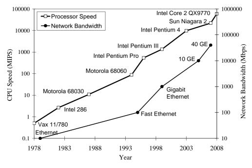
Figure 1.4 Improvement of processor and network technologies over 30 years.
