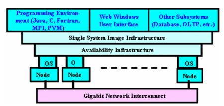
Figure 1.10 The architecture of a working cluster with full hardware, software, anAd middleware support for availability and single system image.
