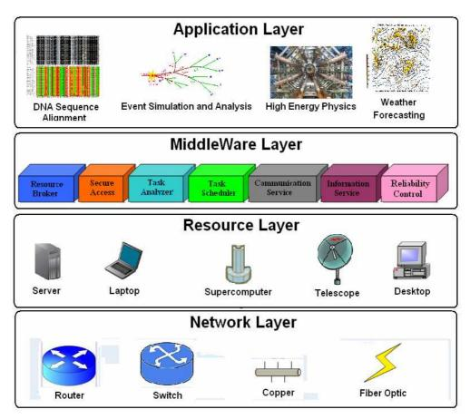
Figure 1.22 Four operational layers of distributed computing systems
